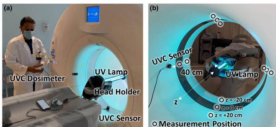
**FIG. 1.** Experimental setup for UV-C dose measurement in a computed tomography scanner gantry. (a) Arrangement of the lamp (suspended from a head holder) and sensor within the gantry. The operator controls the lamp via remote control and reads the dosimeter safely from outside line-of-sight to the lamp. (b) Illustration of 12 sensor measurement positions within the bore — at 4 cardinal locations at  $z = -20, 0,$  and  $+20$  cm from the central scan plane.
