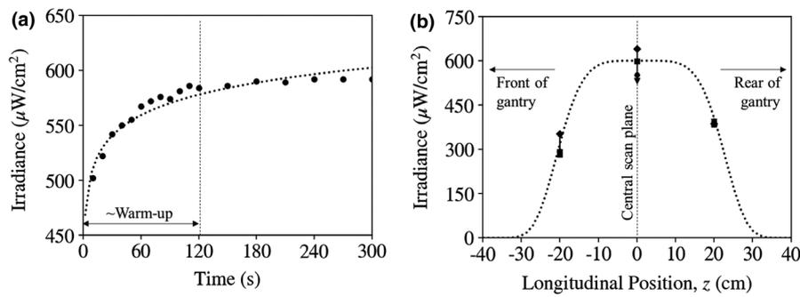
**Fig. 2.** Irradiance measured for the UV-C lamp at a distance of 40 cm. (a) Irradiance measured versus time from switching the lamp on, suggesting a warm-up time of  $\sim 120$  s. (b) Irradiance measured as a function of  $z$  position within the gantry, with negative or positive  $z$  denoting the front or back of the gantry, respectively. The error bars and multiple plot symbols at a particular  $z$  position correspond to measurements at four cardinal locations within the gantry.
